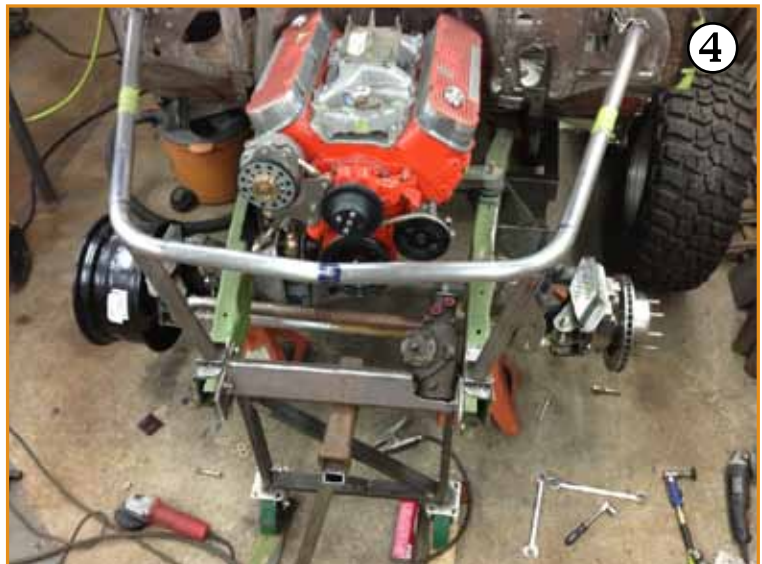
1 - 1972 Blazer before Greg's project started in 2008. 2 - Firewall of Blazer after engine removal. 3 - New handmade parts required Greg to train himself in welding. 4 - Big new V-8 engine. Roll cage tubing, and front axle assembly were designed and built in the garage. 5 - Greg's 4 yr old son, Charlie, poses on the engine.(the next generation!)
